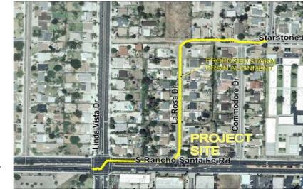
**Justification:** Improve drainage conditions in the west City area at La Rosa Drive, extend storm drain to Rancho Santa Fe Rd and replace old corrugated metal pipe storm drain at Rancho Santa Fe Rd/Linda Vista Drive intersection.
