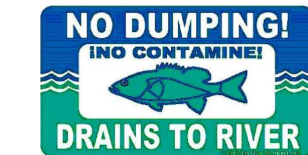
DETAIL "NO DUMPING" AT CATCH BASINS NOTE: ALL CATCH BASINS WITH GRATES SHALL BE STENCILED WITH CITY REQUIRED ITEM PER ABOVE DETAIL (DAS MANUFACTURING #SDO OR EQUIVALENT).
