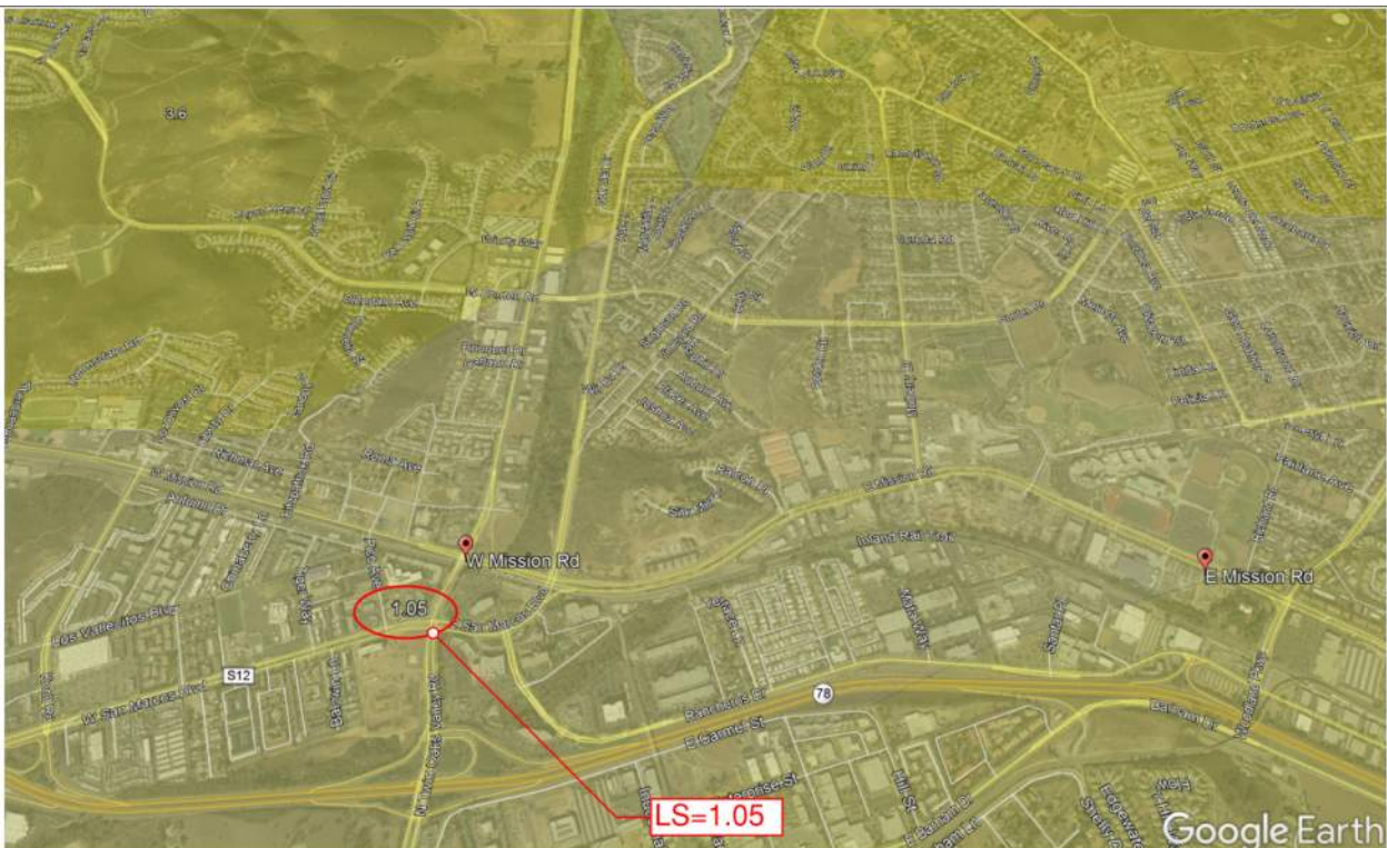
Figure provided from Google Earth with an overlay for RUSLE from SAN GIS LS = 1.05
