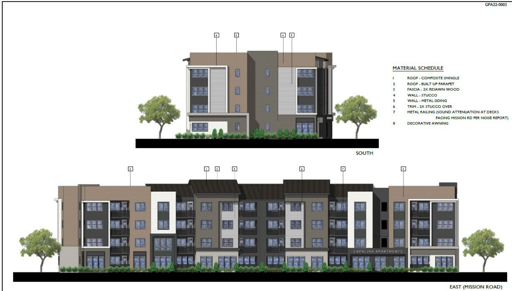
Figure 2-6b. Building B – South and East Elevation
