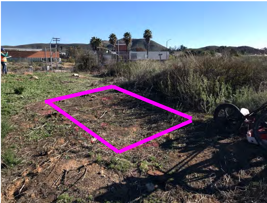
Pink outline shows location of possible UST. Thick vegetation prevented GPR from scanning additional area.
