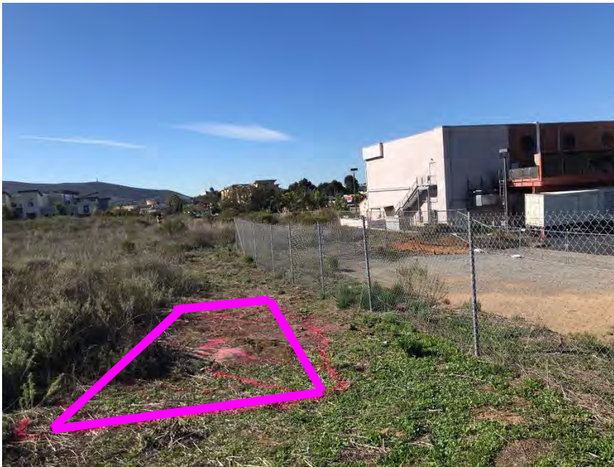
Possible location of UST marked in pink. Fence and vegetation limited GPR scan length.
